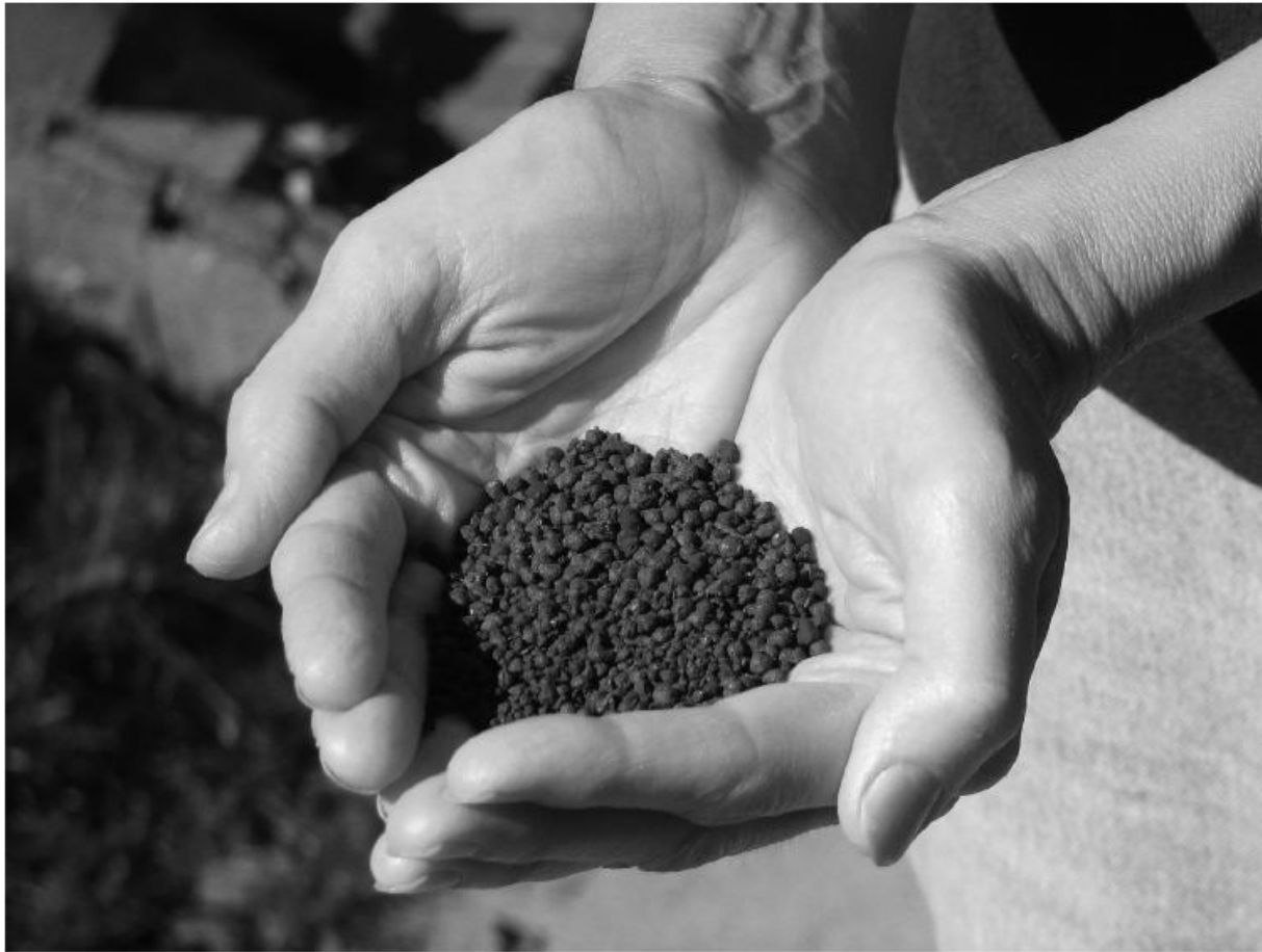
FIGURE 7.8 Treated sewage sludge, shown here in pellet form, is often used as a fertilizer.
