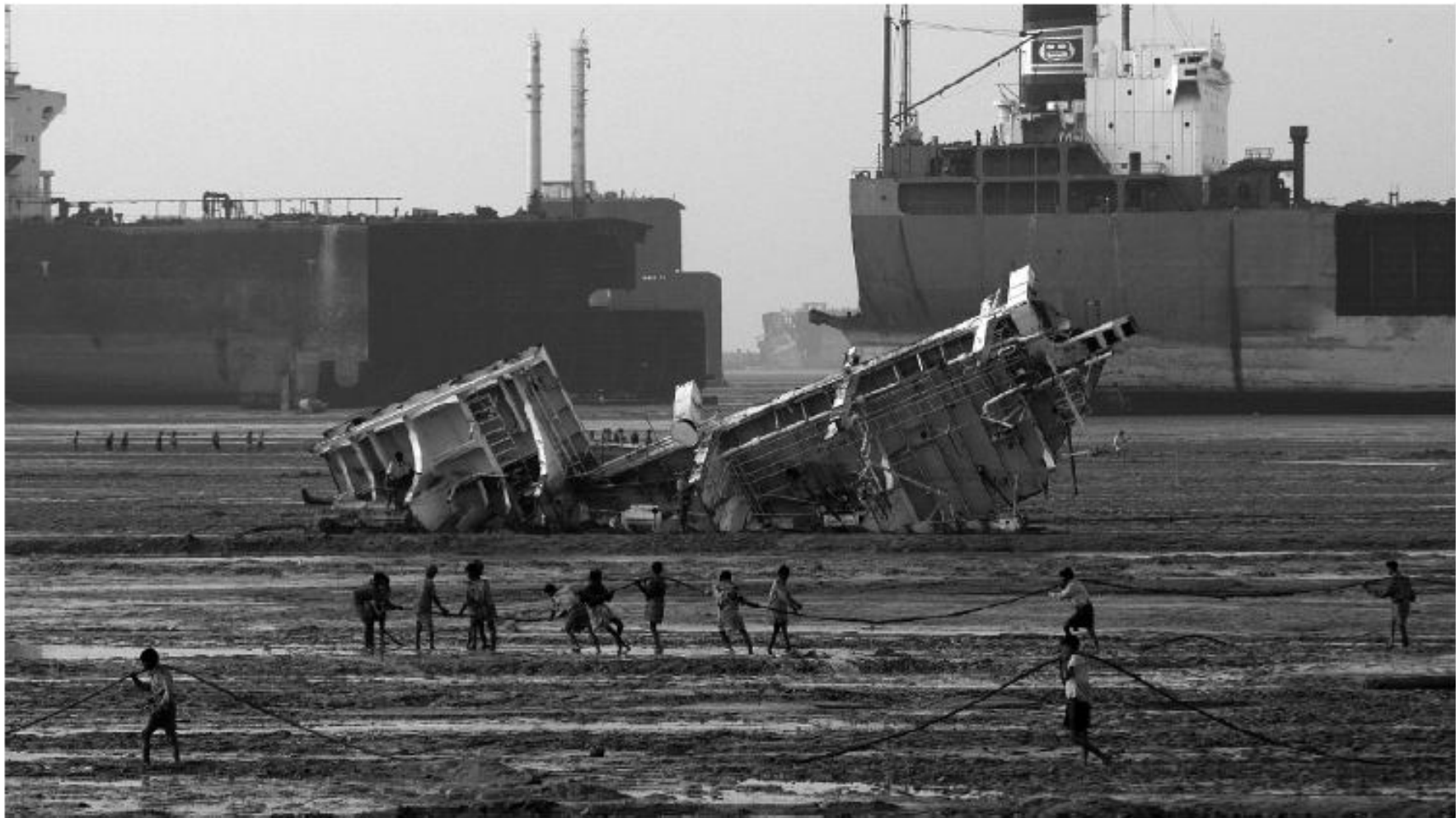
FIGURE 5.7 Manual laborers break down beached ships on the shore of Bangladesh. Source: © 2008 Pierre Claquin. Used with permission.
