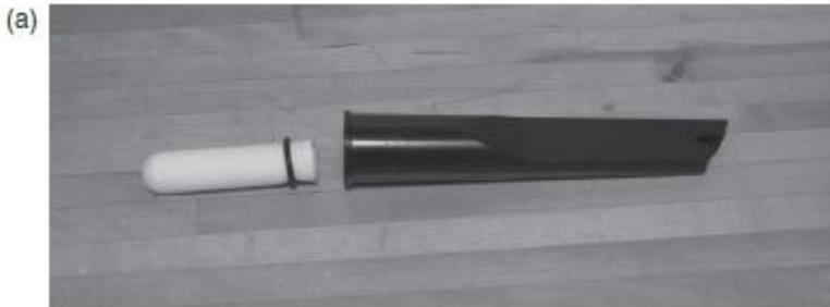
Figure 2.13 Area monitoring: A filter inserted into the nozzle of a vacuum cleaner (a) collects dust to be analyzed in a laboratory. Personal monitoring: A portable sampling device (b) incorporates a pump that takes a continuous air sample near the subject's breathing zone; the device also collects a sample of particulate matter over the whole period.
