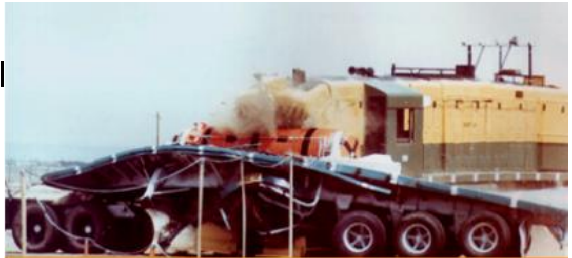
Transportation casks must pass rigorous safety tests before being certified.
