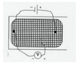
Place the Graph Paper on a table and center the baking dish on the grid. Put 2 or 3 inches of water in the dish and stir in about a half teaspoon of salt. Hook one alligator lead to the positive terminal of the battery pack and the other alligator lead to the negative terminal. Attach each of the wire ends to one of the lead weights and place the weights on opposite sides of the dish.
