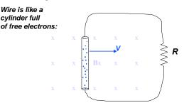
**Example: Find the force required to** move the segment at velocity, v.
