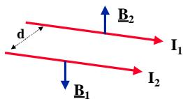
Current 1 produces a magnetic field  $B_1 = \mu_0 I_1 / (2\pi d)$  at the position of wire 2.
