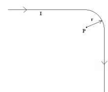
Example: Find the Magnetic Field,  $\mathbf{B}$ , at the point P. The very long wire show carries a current  $I = 5 \text{ A}$  and makes a  $90^\circ$  turn of radius  $r = 5 \text{ cm}$
