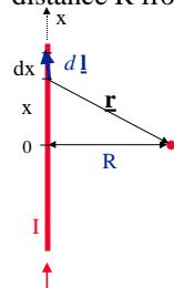
Break the wire into bits  $dl$ . To do that, choose coordinates: let the wire be along the x axis, and consider the little bit  $dx$  at a position  $x$ .
